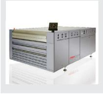
Compact all-in-one system, includes exposure unit for back, main and post exposure, batch-washer, dryer and light finisher. Perfect for narrrow and mid web applications. 24 memory channels for processing parameters and PLC control. Exposure with high power lamps, cooled bed and airflow. Batch washer with solid content measurement and automatic solvent replenishment. Drying section includes four drawers with individual timers.
