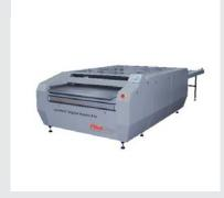
Digital washer with flat and round brushes in large format. Equipped with double tank which allows to separate the black layer of the digital plates from the washout solvent. Automated brush height setting for optimum brush pressure according to the plate thickness. Temperature control of the washout solvent and integrated solid content measurement.
