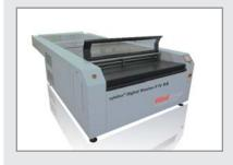
Automatic flowline processor with double tank system to allow separation of digital black layer from washout solvent. Unique washout system with rotating brushes and double lateral alternate oscillating movement. PLC control with colour touch screen display. Specific maintenance program in software. Integrated solvent heater/chiller and solid content measurement with automatic replenishment.
