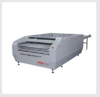
Digital washer with flat and round brushes in mid-size format. Equipped with double tank which allows to separate the black layer of the digital plates from the washout solvent. Automated brush height setting for optimum brush pressure according to the plate thickness. Temperature control of the washout solvent and integrated solid content measurement.
