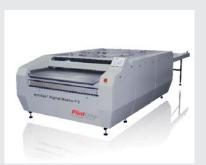
Digital washer with flat and round brushes in large format. Equipped with double tank which allows to separate the black layer of the digital plates from the washout solvent. Automated brush height setting for optimum brush pressure according to the plate thickness. Temperature control of the washout solvent and integrated solid content measurement.
