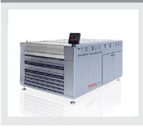
Compact all-in-one system, includes exposure unit for back, main and post exposure, batch-washer, dryer and light finisher. Perfect for narrrow and mid web applications. 24 memory channels for processing parameters and PLC control. Exposure with 16 high power lamps, cooled bed and airflow. Batch washer with solid content measurement and automatic solvent replenishment. Drying section includes four drawers with individual timers.
