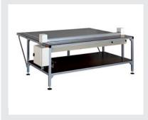
Designed for the cutting of foil based polymer plates up to 7 mm plate thickness (before and after processing). The cutting blade and clamp is operated by compressed air. With illuminated cutting channel for best cutting accuracy, cutting angle 90 °. With two-handed operation for optimum work safety.
