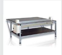
Designed for the cutting of foil based polymer plates up to 7 mm plate thickness (before and after processing) . The cutting blade and clamp is operated by compressed air. With illuminated cutting channel for best cutting accuracy, cutting angle 90 °. With two-handed operation for optimum work safety.
