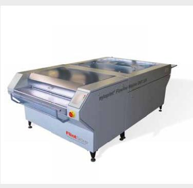
A tankless flowline system, offering water washout, drying and post exposure all in-line. A touch screen display offers easy operation, including control of the water temperature and flow speed. The proven, plush' system that is easily adjustable, provides optimum washout results. Includes automatically lowering squeegee roll, adhesive carrier plate for foil based plates and magnetic carrier plate for metal based plates.
