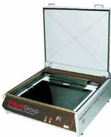
A washout system for the production of alcohol washable nyloprint® printing plates. The washout unit features a proven plush pad as well as an oscillating plate holder and includes an adhesive and magnetic carrier plate for use with foil and metal based plates. User-friendly details such as the count down facility, audio alarms notifying the user of the end of the process.
