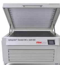
Premium quality system for main and post exposure as well as drying of nyloprint® printing plates with integrated chiller. It includes four drawers and 20 memory programs for main and post exposure. Operation of each tube is monitored and operating hours of tubes are recorded.
