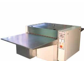
A flowline system for the optimum production of alcohol washable nyloprint® printing plates. The system provides washout, rinsing, post cleaning and pre-drying all in one device. A closed continuous system in an explosion proof protected design. Washout speed is easily adjustable via a digital display. Washout solvent is controlled to ensure a constant temperature. The height of the plush carriers can be easily adjusted to suit different plate thicknesses.
