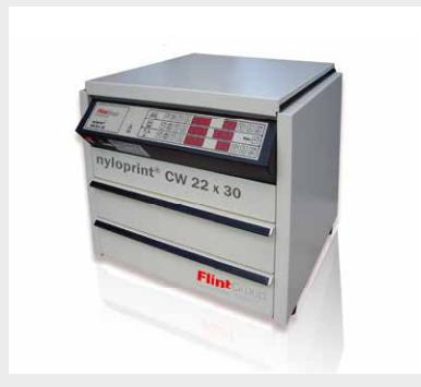
The smallest of the equipment combinations is a space saving, 'all-in-one' plate making device. It is equipped with an oscillating, self-adjusting plush washout system, horizontal exposure and a drying drawer. Includes adhesive and magnetic carrier plate for use with foil and metal based plates and a digital display for easy use.
