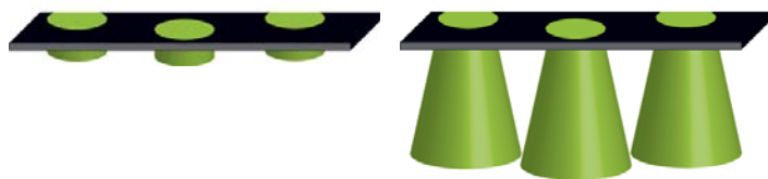
Step 1 – High intensity UV surface crosslinking
