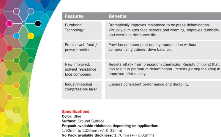
Metal Backing: 0.20mm Stainless Steel Backing Face Compound: Solvent Resistant Rubber Blend
